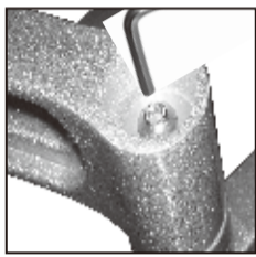
Fig. 6 - Use the Alley Key to tighten the arms and prevent unwanted movement.
